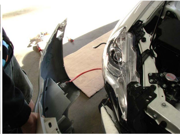
Notice a wire connects the bumper to the car
