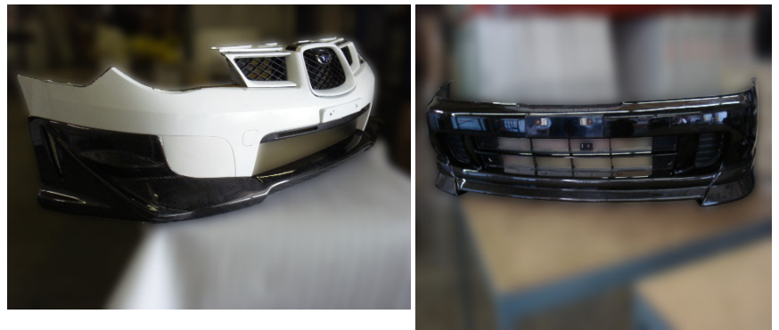
Fig. 10 Now that all final adjustments have been made to secure the lip, the bumper can be reinstalled on the car.
