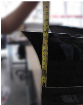
Fig. 5 After adjustments are made, properly align the lip onto the bumper. Measure both ends, make sure they are of equal heights and that the lip is snug. Keep lip in place with masking tape.
